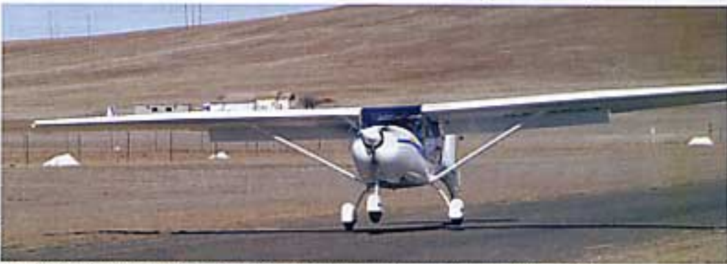
The wing of the Allegro has a huge 10.8 metre span, providing for very large ailerons without sacrificing flap area.
