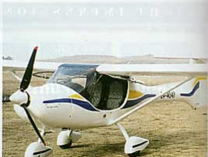
Power is provided by a Rotax 4 cylinder 4 stroke 912S, developing 100hp (75kW) and driving a three bladed Woodcomp composite propeller.
